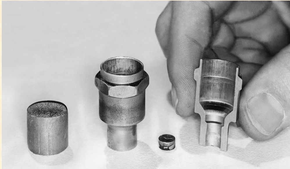
Figure 15.12 Production steps for a cold extruded spark plug.
